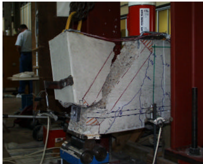
Figure 6-2: Failure of specimen CCT-08-45-10.39-2
